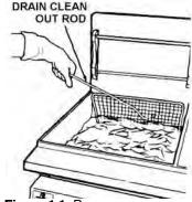
Figure 1.1: Remove screen over elements/ tubes
